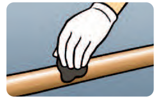
APPLY EPOXY PUTTY
